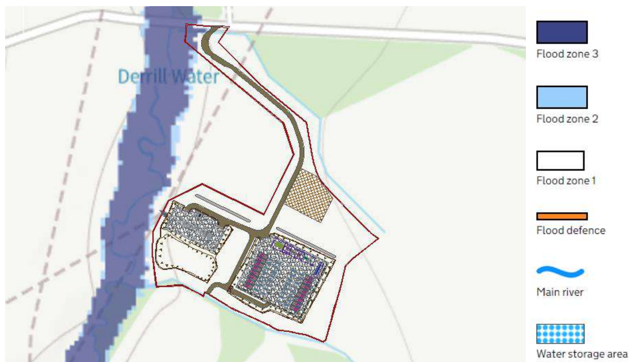
Figure 2 - Excerpt from the Environment Agency fluvial flood risk map, with proposed development overlaid
