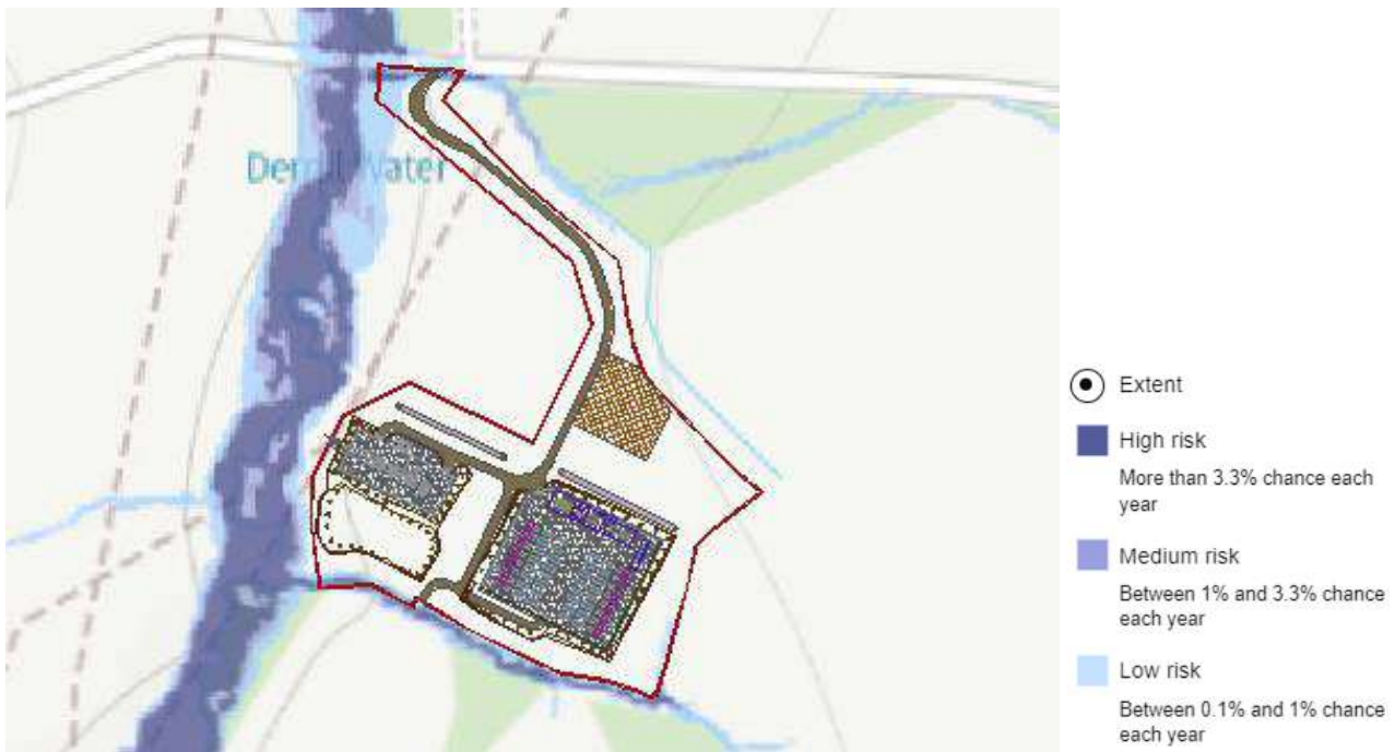
Figure 3 - Excerpt from EA surface water flood risk map, with proposed development overlaid
